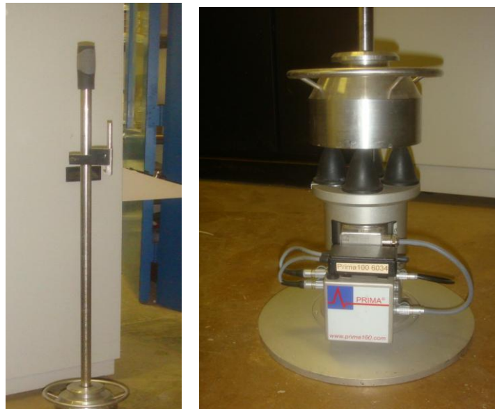
Figure 3-32 PFWD release trigger (Left) and drop weight, rubber buffers, velocity transducer (Right)
