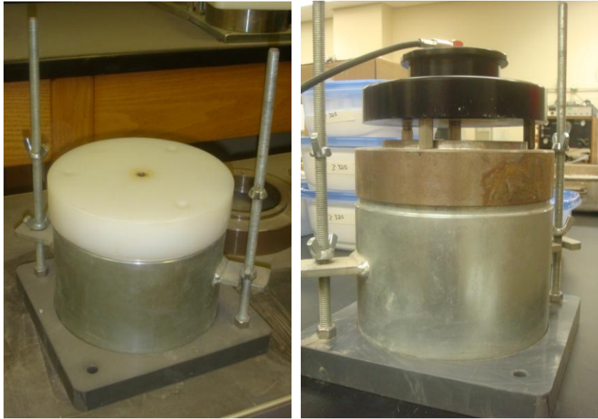
Figure 3-17 Center rod guide and non-conductive base (Left) and coaxial head and mold collar on compaction mold (Right)
