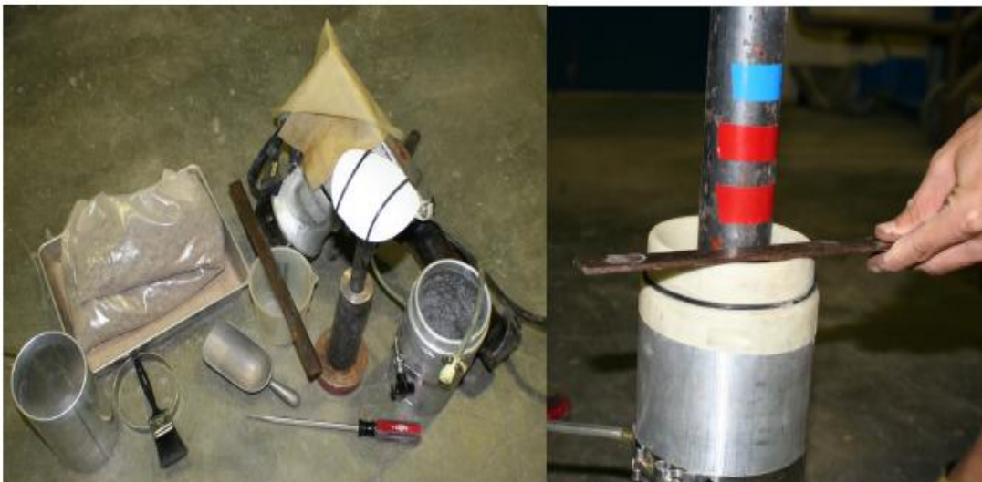
Figure 2-25 Sample preparation apparatus (left) and compaction density control (right)
