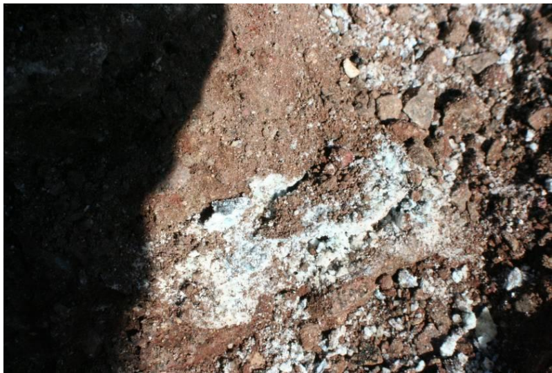
Figure 5.1 (a) and (b) Pavement eruptions; (c) and (d) White reaction product found in the base course
