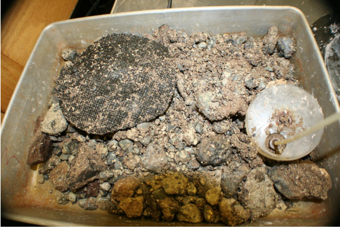
Figure 4-10 100% RCA (subbase gradation) or Sample 3 after 95 days of CO 2 bubbling showing no appreciable tufa precipitate
