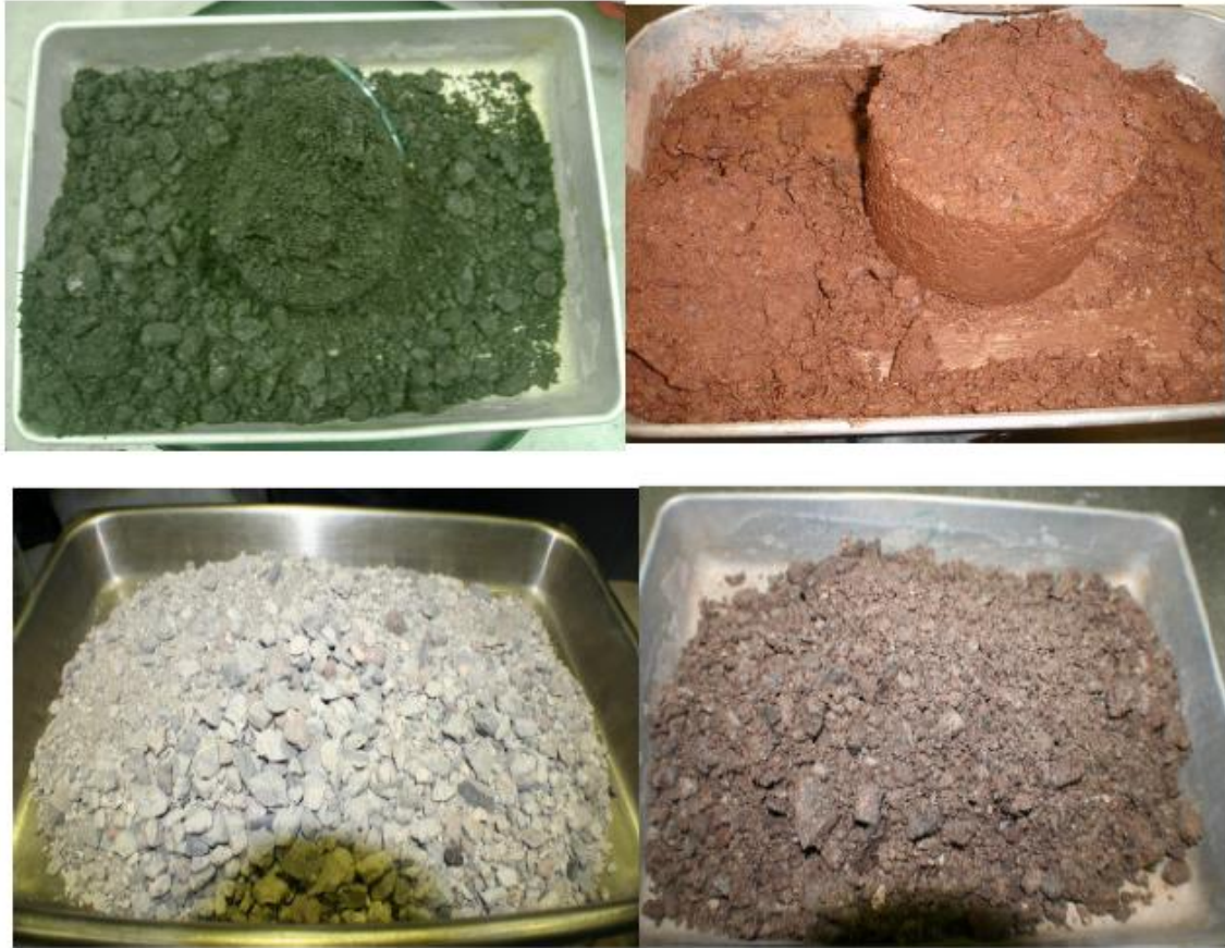
Figure 2-24 Materials tested: RAP after M_r testing (top left), RG and VA blend after M_r testing (top right), 100% RCA before (bottom left) and after (bottom right) mixing with water but before M_r testing.
