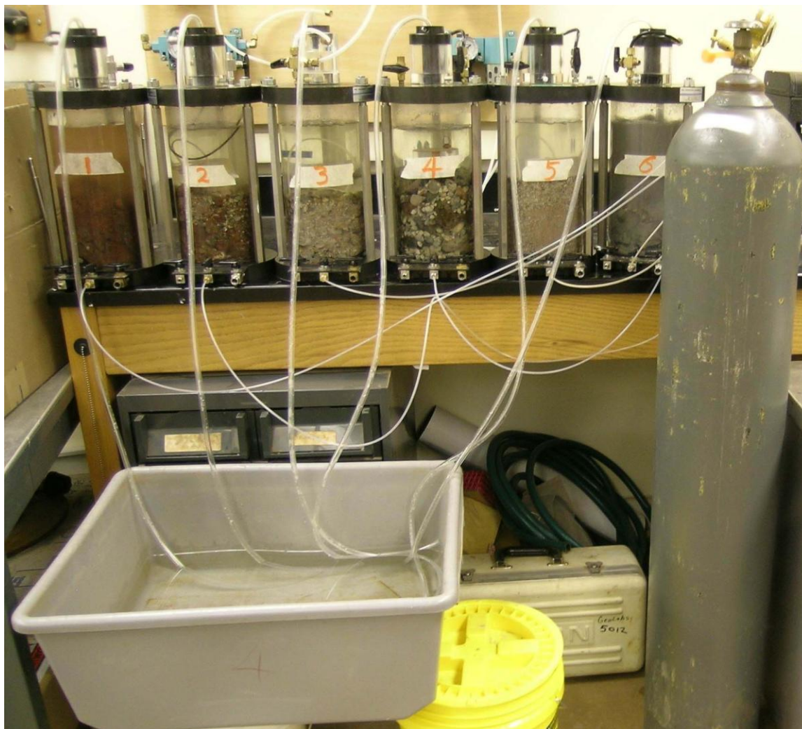
Figure 4-1 Test setup for bubbling CO 2 through RCA soaked in rain water. CO 2 is fed through the bottom of each test chamber. It then bubbles up through the aggregate solution and exits at the top of the chamber into a hose that feeds into the large plastic container filled with water
