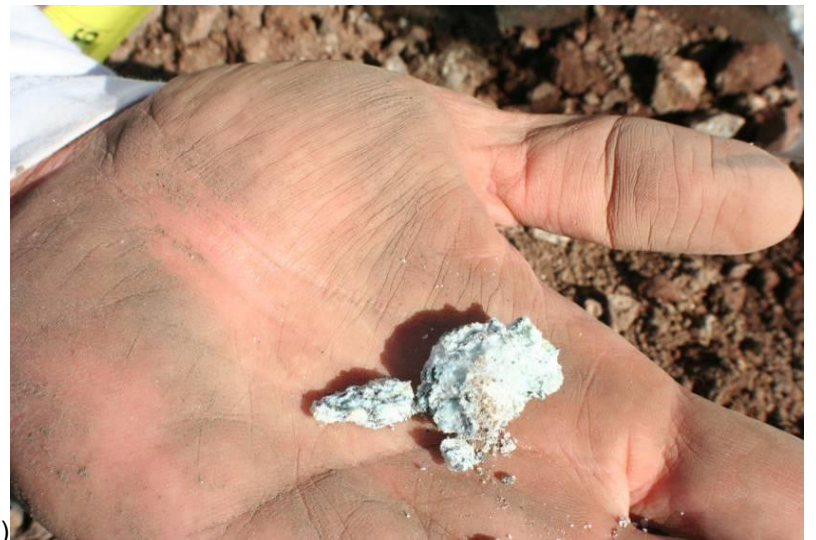
Figure 5.1 (a) and (b) Pavement eruptions; (c) and (d) White reaction product found in the base course
